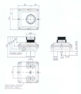
FOR A ACTUATOR SHAFT HEIGHT OF 20mm - A = 28mm FOR A ACTUATOR SHAFT HEIGHT OF 30mm - A = 18mm NOTE FOR A ACTUATOR SHAFT HEIGHT OF 20mm - A = 28mm FOR A ACTUATOR SHAFT HEIGHT OF 30mm - A = 18mm
